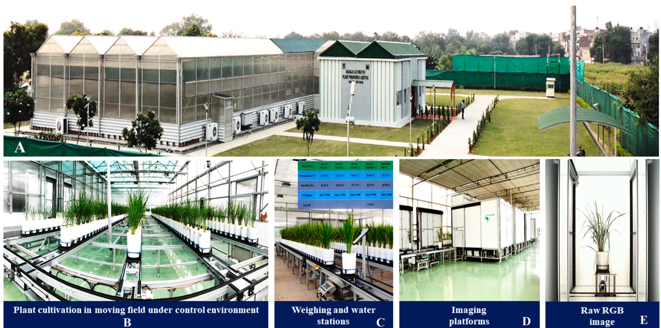
Fig. 1. Nanaji Deshmukh Plant Phenomics Centre (NDPPC), ICAR – IARI, New Delhi, India. (A) Panorama view of the Centre; (B) Plants are grown in a greenhouse with conveyor belts; (C) Movement of plants in an automated system and weighing and watering. (D) Imaging chambers to capture different types of data, (E) An example of the side view RGB image of a rice.
