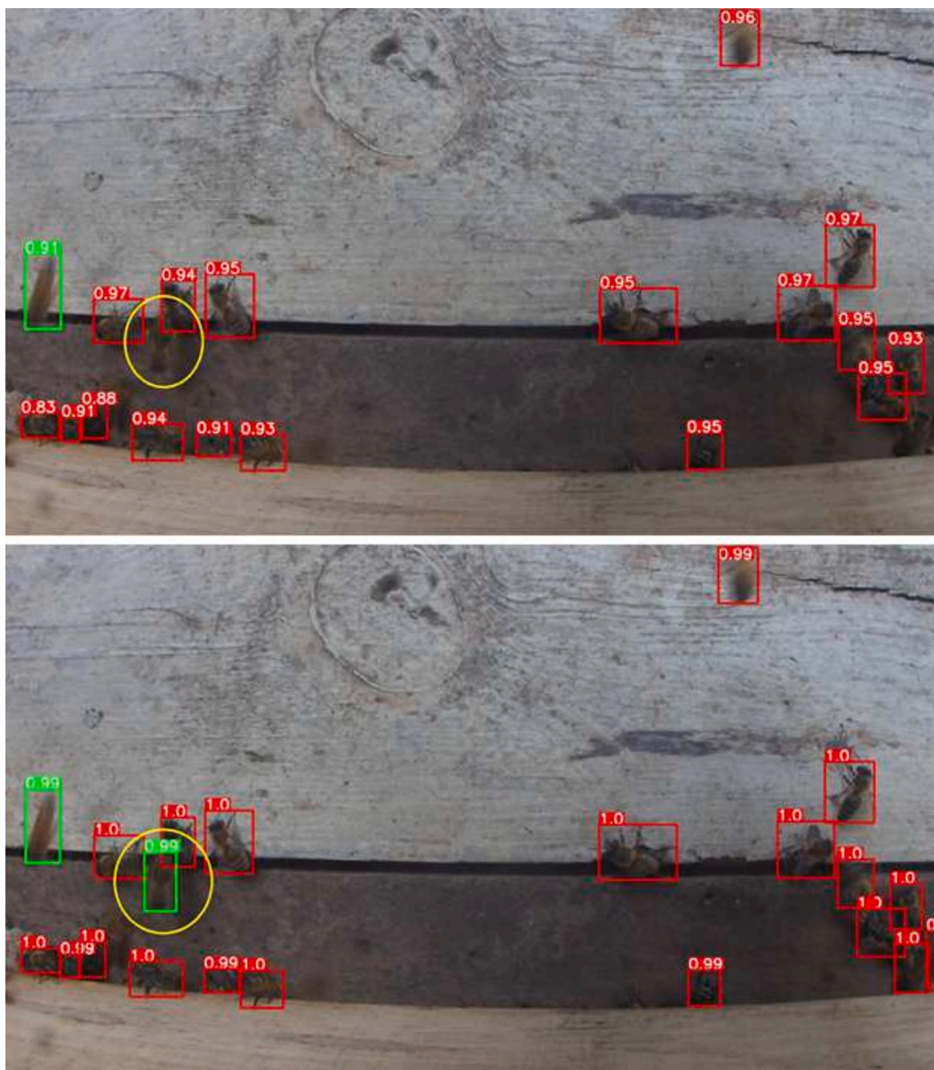
Fig. 15. Detection results of the proposed improvement: (above) YOLOv5 + focal loss, (below) Faster RCNN + Overlap sampler. The green and red boxes indicate pollen-bearing and non-pollen-bearing bees, respectively. Values indicate the confidence score. (For interpretation of the references to color in this figure legend, the reader is referred to the web version of this article.)
