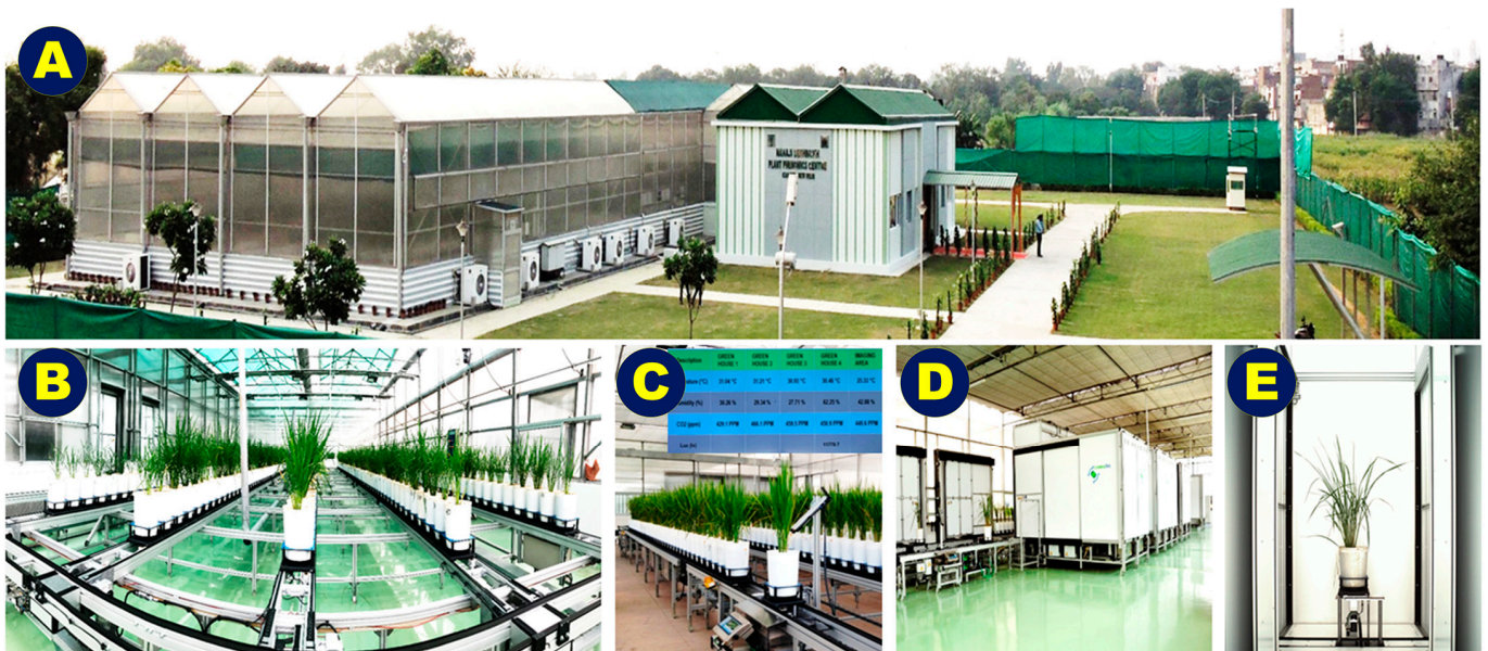
Figure 1. Experimental set up at Nanaji Deshmukh Plant Phenomics Center (NDPPC), ICAR—Indian Agricultural Research Institute, New Delhi, India. (A) High-throughput phenotyping (HTP) facility comprises four climate-controlled greenhouses, an imaging area and server room, and an admin block. (B) Pot culture experiment in the climate-controlled green-house; (C) automatic weighing and watering station; (D) imaging area with chambers installed with RGB, IR, and NIR cameras to acquire top- and side-view images. (E) RAW images were acquired from a side perspective view at 0° angle.
